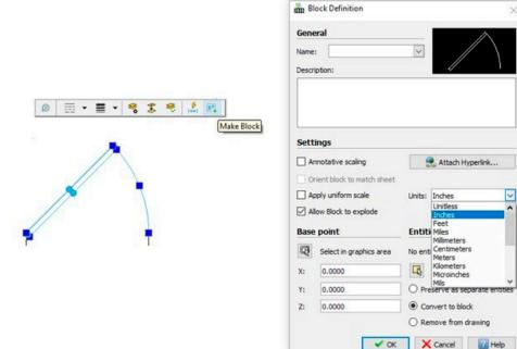
DraftSight also supports inserting and manipulating AutoCAD Dynamic Blocks. You'll be able to access all the actions and parameters as you always have.
